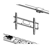
Screen mount incorporated into the housing backplate.
